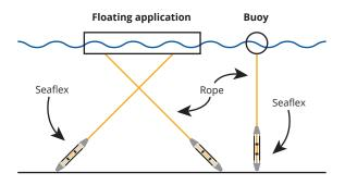
SEAFLEX is used whenever there is a need to anchor something floating, such as commercial marinas, wave attenuators, floating solar parks or wave energy converters. The system expands and retracts with each tide and wave, taking on and dampening the forces year after year.
